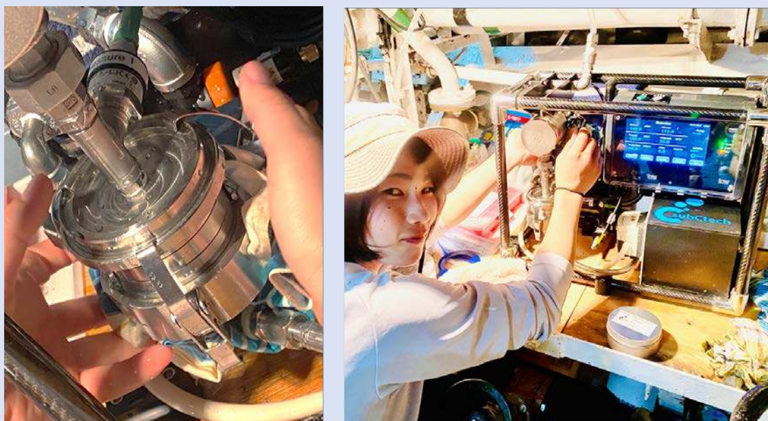
Figure 2 Filters of the semi-automatic microplastics sampler (left); and Yurie Seki working on the microplastic sampler (left) changing the filters to collect the microplastic samples (right)
