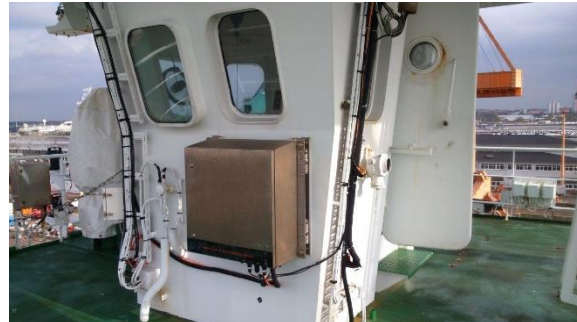
Additional "Top-Box" with independent air CH 4 analyzer, GPS and interfaces to meteo sensors. Simple data interface to the OceanPack™ system.
