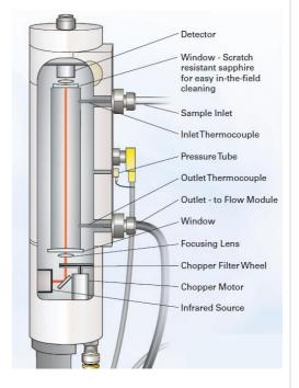
resistant sapphire, allowing for worry-free cleaning in the field. (Image & Text © LI-COR\*)
